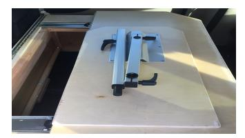
3. By using the handles and pressing the button, loosen and slide the leg down to remove the detachable leg for the table.
